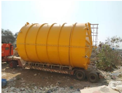
150KL –HCL Storage Tank
